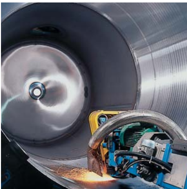
Our internal grinding machine for bodies, dished ends and nozzles works entirely automatically. Perfectly ground steel surfaces form the ideal substrate for the glass-lining
